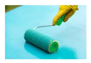
PreTreat TACKY OVEN COATING is a polymeric based coating formulated for use in high temperature paint ovens. This product is applied to a sheet of steel or aluminium, wrapped in aluminium foil, by a paint roller. Then passed through the oven to trap air borne particulates that may otherwise be deposited on freshly painted surfaces. PreTreat TACKY OVEN COATING remains tacky for extended periods of time at temperatures up to 250° C.
